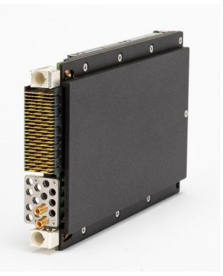
The VPX Timing Clock offers a complete solution set for all PNT needs. This highly ruggedized conduction cooled unit provides a versatile multifunction clock references for any environment.
