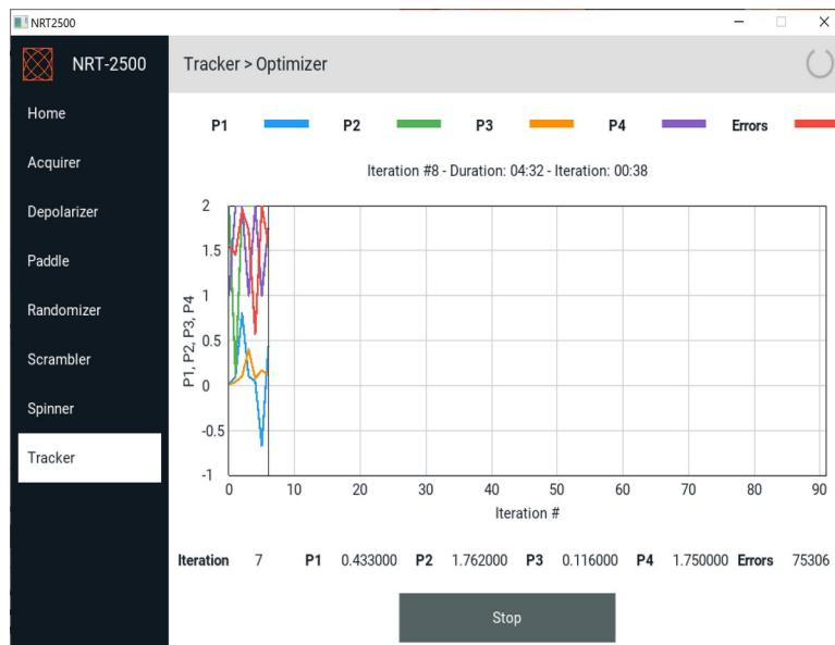
*Figure 22: TEF Optimizer step 4 - While the optimizer is running, the set of 4 optimization parameters is displayed together with the number of tracking errors measured. Each iteration value can be viewed in the Iteration Data box. Terminate the execution of the Optimizer program by clicking on any of the 3 buttons below the graphic screen.*
