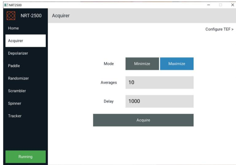
*Figure 43: Acquirer Mode: Once the Acquire button is pressed, the unit will adjust the SOP to acquire the minimum or maximum value of the TEF. The number of Averages, and Delay time between the SOP update and a measurement of the feedback are set by the user.*
