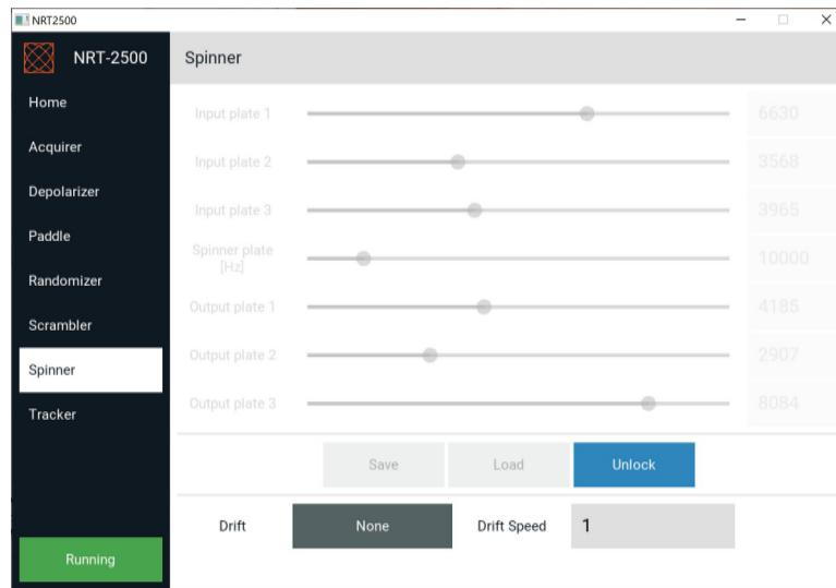
*Figure 29: The Drift mode will read None (no drift). Press on the Drift button to select the desired drift mode. Choose between None, Along Spin Axis, Rotate Spin Axis or Both (see Figure 30). You can also change the drift rate between the non calibrated drift rates 1-10.*
