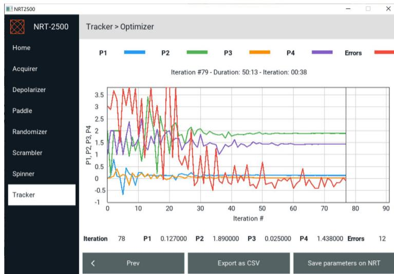
*Figure 23: TEF Optimizer step 5 – once the Optimizer execution is terminated, the 4 optimized parameters are shown in the lower part of the window. The user may choose between 3 options:
