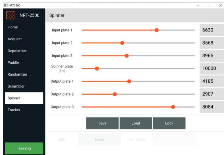
*Figure 28: You can now change the sliders positions. Pressing the Load button will restore the values to the values saved before the changes have been made. Pressing the Lock button, the plates sliders and indicators as well as the Save and Load buttons will be grayed out and locked. The Drift mode selector and speed will appear on the bottom of the GUI window (see Figure 29).*
