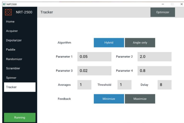
Figure 13: Once the communication between the computer ant the NRT-2500 was established the NRT-2500 will default to Tracker Mode and the tracker screen will show up. The values showed by the GUI are the last values that were used in the GUI.
