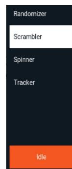
Figure 25: Stop the Scrambler execution by clicking on the RUNNING indicator. The indicator will turn amber and read IDLE. (You may also set the  $R_{mode}$  speed to 0 to stop the Scrambler.)
