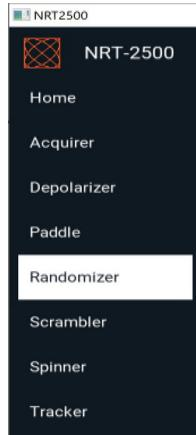
Figure 15: The Mode Selector bar. Click on the mode you would like to select, the GUI screen will adjust to the selected mode.
