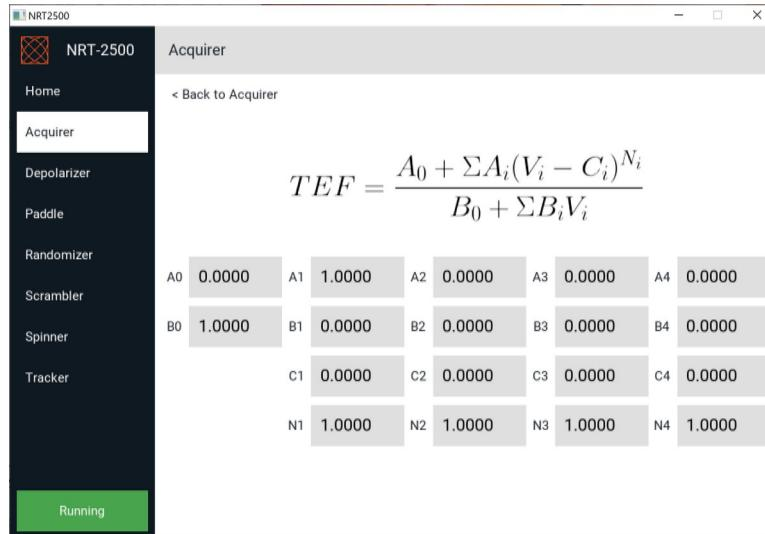
*Figure 44: Acquirer Mode TEF: The TEF for the Acquirer mode is the same TEF used in the Tracking mode. Above is the most common TEF measuring the voltage (usually from a photodiode), measured at BNC 1 on the rear of the NRT-2500.*
