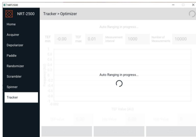
*Figure 19: The TEF Optimizer – Step 1, Auto Range: the unit will auto range the input level of the Tracking Error Signal and acquire a histogram of that signal to visualize the system behavior and allow the user to better define the level at which the system would be considered to be below the desired...*
