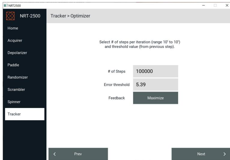
*Figure 21: TEF optimizer Step 3, Select the number of steps per optimization iteration. Confirm the value of the Error Threshold, select Minimize or Maximize the TEF. and then press OK to start the Optimizer execution.*
