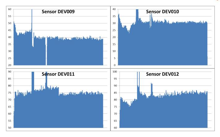
Some of the noise in the early part of the run is due to fluctuations in the chamber cycle as can be seen below:
