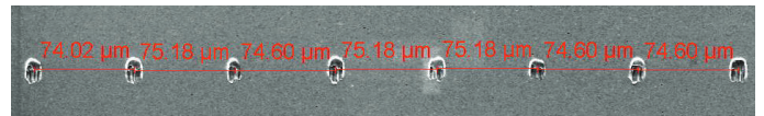
Figure 12. Probe marks of InfinityQuad showing X & Y errors of less than 1\ \mu\text{m} at ambient temperature.
