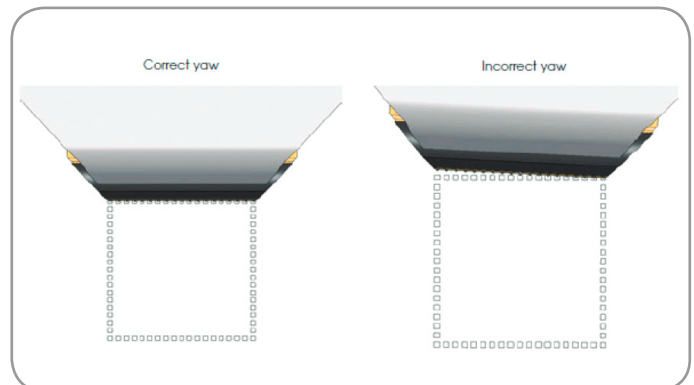
Fig 8. Effect of incorrect yaw alignment
