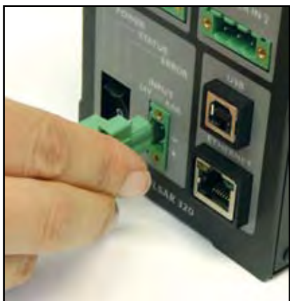
Figure 2: 24v Supply Connection
