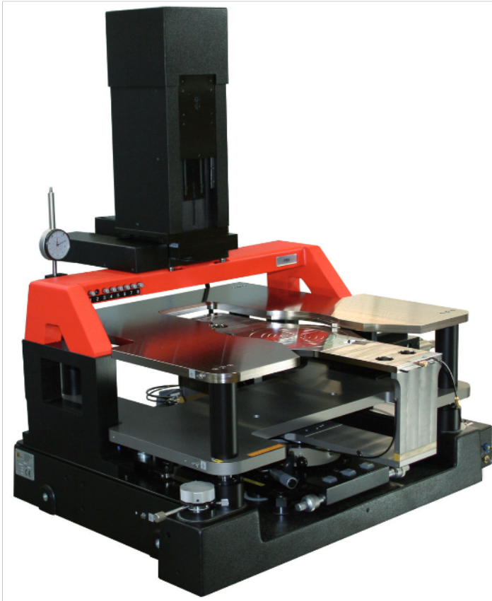
Setup prepared to integrate an OEM emission microscope camera system onto the microscope bridge.
