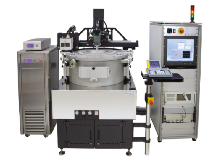
PAV200 with Black Body for microbolometer testing.
