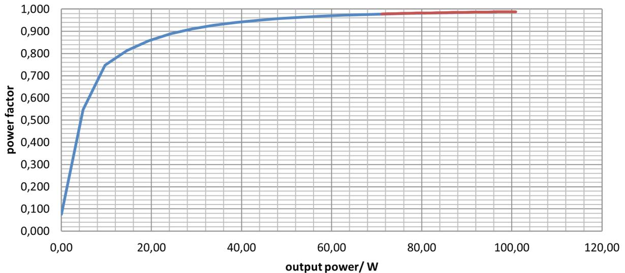
— power factor vs output power at const output voltage
