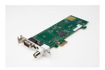
The PCI-Express SyncClock LP from Brandywine Communications provides precision time with zero latency to the host computer over the PCI bus. An on-board microprocessor automatically synchronizes the clock to reference signal inputs. The reference signal inputs can be 1 PPS, IRIG or NASA time codes and optionally, GPS or HaveQuick. The clock can free run and be set by commands from the host over the PCI Express bus.
