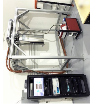
Model 119 Overhead Stand. Dimensions: 1.5m width, 1.23m depth, 2.21m inside height, 2.69m total height
