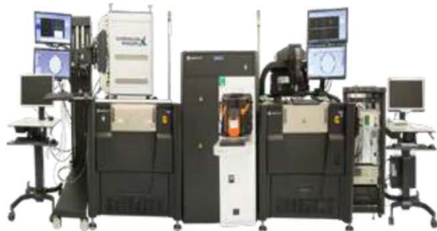
Figure 2: Test system for evaluation of micro-bump probe cards installed in Fab-2 at imec.
