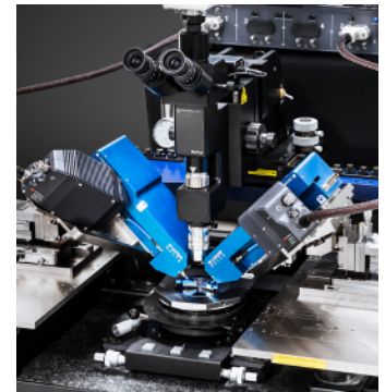
Full integration of VDI mini frequency extenders (left) and Focus Microwave's Load-Pull Delta Tuners (right). The RF arms are equipped with a dove tail that makes it easy, safe and fast to change between different measurement applications.
