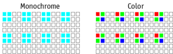
Figure 4: DecimationHorizontal / DecimationVertical = 2. 2x reduction factor. 2 of 4 columns/rows displayed
