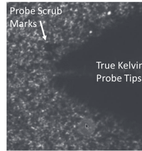
(a) True Kelvin Probes on Contact Substrate for Probe Planarization
