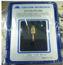
(b) True Kelvin DC probe with pitch 8 \mu\text{m} , probe tip radius of 1.5 \mu\text{m}
