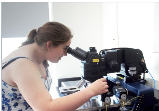
Figure 2: A student researcher operates a Cascade EPS150FA probe system to acquire data on the electrical behavior of newly synthesized materials.
