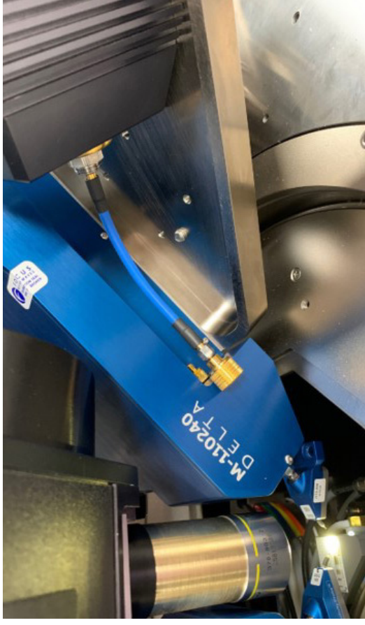
To connect a coax standard to the end of the cable, the Keysight N5291 frequency extender can easily unclamp and slide back via quick release mechanism. The cable is semi-rigid and provides highest phase stability.
