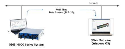
The 3DViz software maps and displays live strain and temperature data streamed in real-time from a networked ODiSI system.
