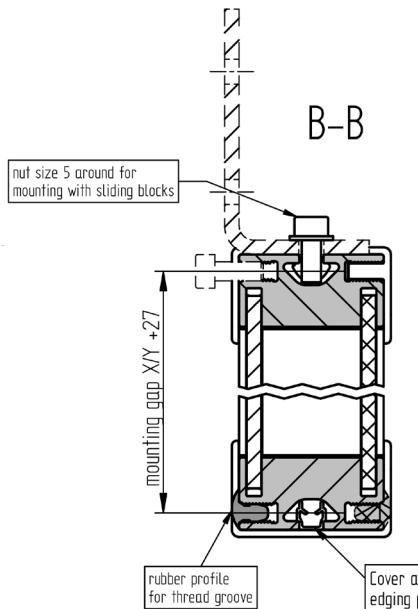
optional cover of the surrounding M4 thread groove using a cover profile to protect against dirt and dust
