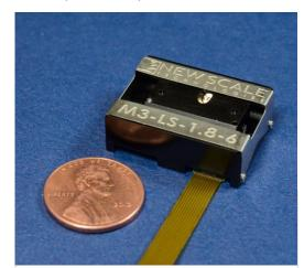
**The M3-LS Linear Smart Stage** is an ultra-compact positioning stage with high resolution, low power use and absolute encoding. All electronics are built into the stage for simple system integration. Control the stage using high-level motion commands via USB, I<sup>2</sup>C or SPI interface.
