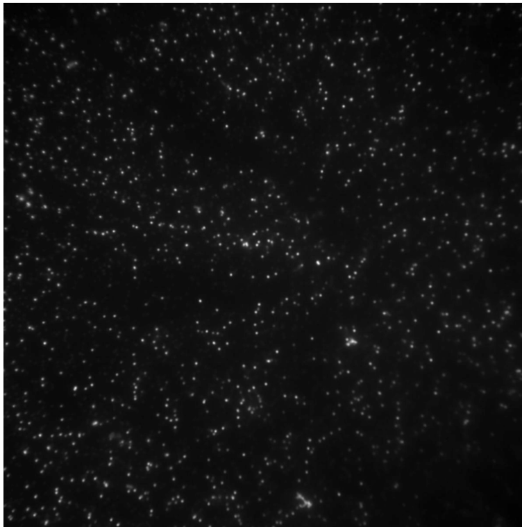
Figure 1 Alumina ( \text{Al}_2\text{O}_3 ) coated gallium phosphide (GaP) nanowires functionalized with biotinylated BSA (bovine serum albumin). Streptavidin labelled with three fluorescent dyes (FITC, TRITC and Cy5), imaged under 100x magnification.
