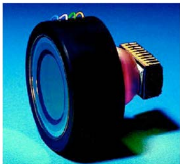
Figure 4. An intensifier coupled to a CCD via a fiberoptic offers the highest possible sensitivity in low-light-level applications.
