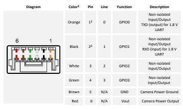
1-GPIO cable assembly wire colors
