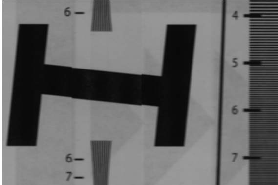
Out-of-focus image with vertical misalignment
