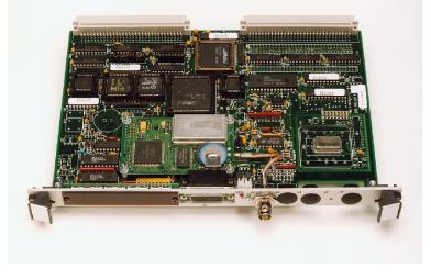
The VME-SyncClock32 from Brandywine Communications provides precision time with zero latency to the host computer over the VME bus. An on-board microprocessor automatically synchronizes the clock to reference signal inputs. The reference signal inputs can be 1 PPS, IRIG A or B and NASA 36 time codes. GPS and Have Quick inputs are optionally available. The clock can free run and be set by commands from the host over the VME bus.
