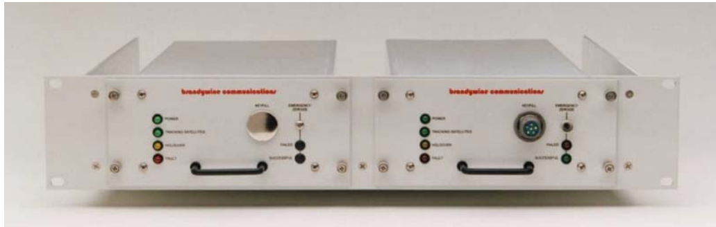
PTS shown with C/A code and SA-ASM GPS in rack mount case
