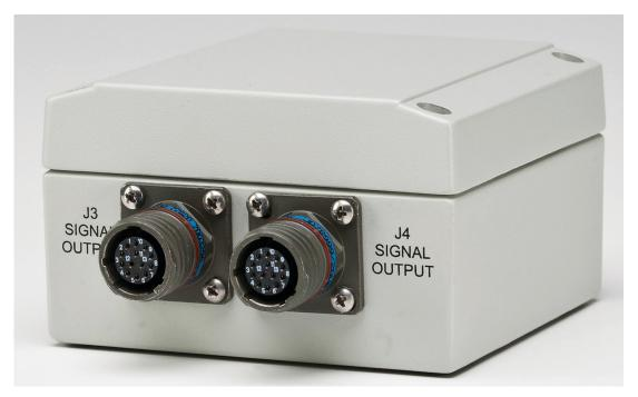
Brandywine Communication's Havequick/1PPS Distribution Amplifier (HQS) is a small rugged, powered Havequick/1PPS distribution module mounted in a 4" x 4" x 2.5" environmentally secure enclosure. The HQS can provide an MTBF up to 1 million hours depending on configuration.
