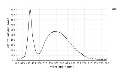
White LED illumination is the most commonly used machine vision lighting configuration. It is often the default choice when specific features of interest do not require color-based highlighting. However, white LEDs can vary in color temperature between different lighting families, , which can impact machine vision systems, specifically when matching white light sources.
