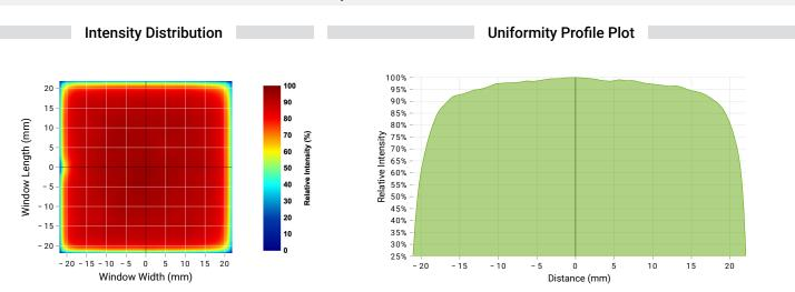
The BL245 Series provides a highly uniform output across its emitting window with an edge effect of only 18.4mm, and a uniformity of +/- 10% within the optical area.
