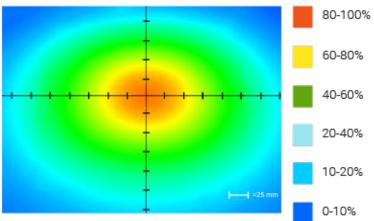
Optical measurement taken using AL116-WHIIC Rev. A @ 200 mm
