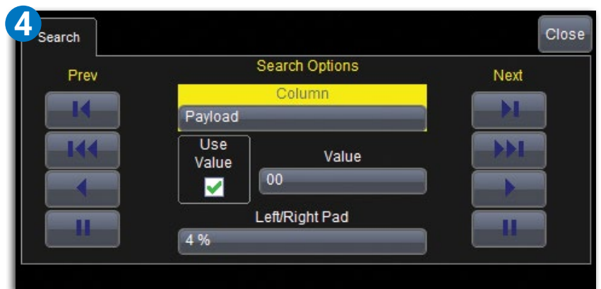
Search can locate up to 14 selectable criteria for DigRF 3G and 18 criteria for DigRF v4, or narrow down the search by entering a value.
