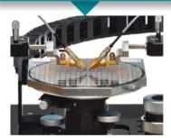
RF chuck with < ± 3 μm surface planarity
