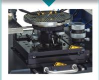
Probe card simultaneously used with single needles (option)
