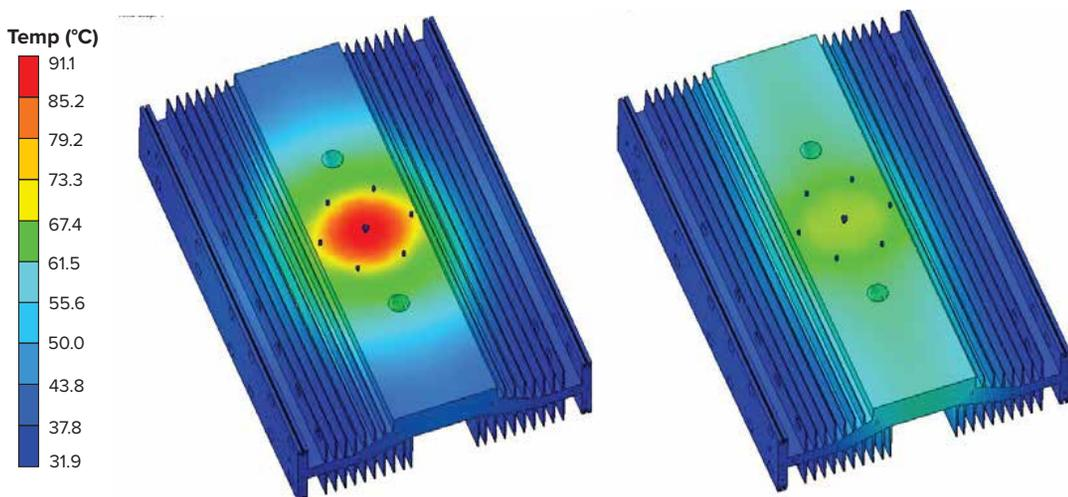
Thermal image of Air Cooled IGBT Heat Sink. Left: no heat pipes. Right: with heat pipes (HiK™)
