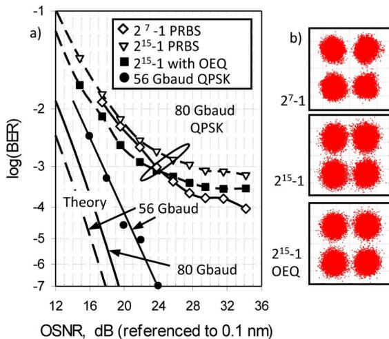
Fig. 5. (a) BER measurements for 80-Gbaud (160-Gb/s) QPSK with and without OEQ; 56-Gbaud data [5], [11] are shown as a reference. (b) Constellation diagrams for PRBS lengths of  $2^7 - 1$  and  $2^{15} - 1$ , the latter with and without OEQ, all measured at an OSNR of 34 dB.
