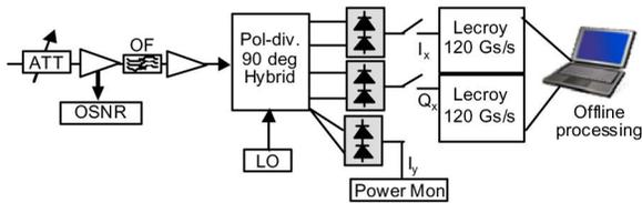
Fig. 3. Single-polarization coherent receiver based on two 120-GSamples/s oscilloscope prototypes with 45-GHz input bandwidth to individually detect the signal's two quadratures.
