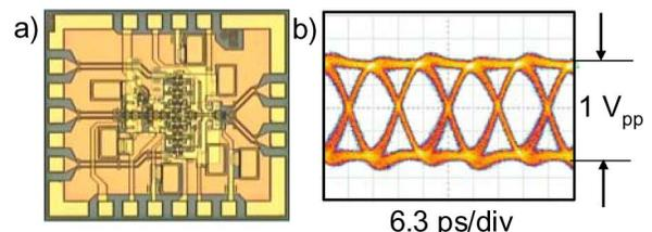
Fig. 2. (a) Microphotograph of the 2:1 InP HBT multiplexer; (b) electrical output eye diagram at 80 Gb/s for a PRBS  $2^{15} - 1$ .
