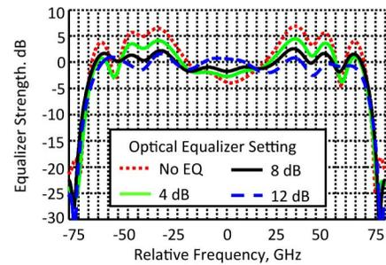
Fig. 7. DSP equalization strength for four different received optically equalized signals with varying OEQ settings.
