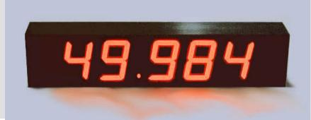
These displays are suitable for interior applications where clearly presented line frequency is required. The displays are single-sided and indicate line frequency to 3 decimal places on 7 segment high intensity LED digits.
