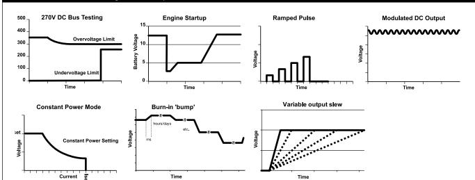
SGI model provides constant power mode allowing independent setting of the max voltage, current and power
