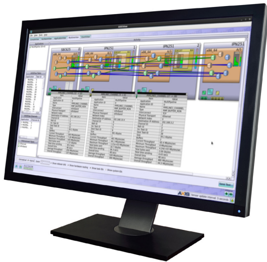
Diagram 4: Task mapping across a 6U OpenVPX multi-board, multi-node CPU/GPU system using InfiniBand and Ethernet.
