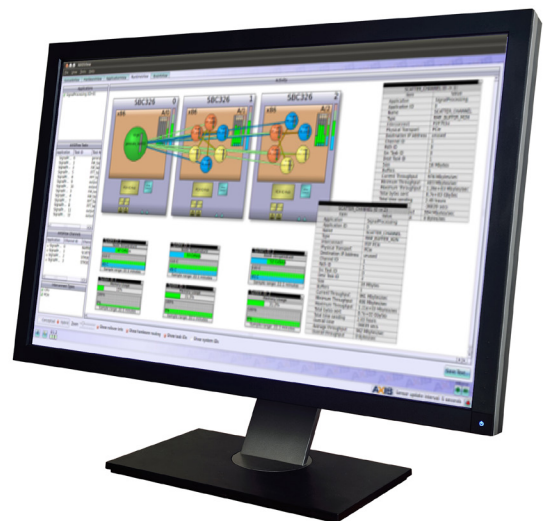
Diagram 5: Signal processing application mapped to a 3U OpenVPX Intel 4th Generation Core-i7 HPEC cluster running VxWorks and using gen 3 PCIe P2P data plane fabric.
