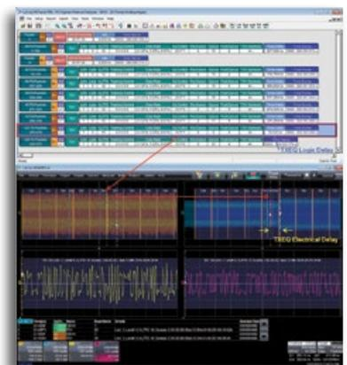
In this example, the PeRT<sup>3</sup> is programmed to negotiate with the DUT during PCI Express 3.0 link equalization training while all worst case electrical jitter sources are calibrated and turned on. The PeRT<sup>3</sup> can then be setup to trigger the oscilloscope based on specific states of the link equalization training. The oscilloscope uses the trigger to capture the upstream and downstream traffic for protocol decode and cross linked protocol and PHY layer analysis.
