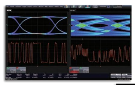
The Teledyne LeCroy SDAIII-CompleteLinQ Serial Data Analysis products contain multi-lane eye and jitter analysis, LaneScape™ comparison modes, vertical noise measurements, and crosstalk analysis tools. These capabilities provide the deepest insight into the behavior of multi- or single-lane serial data systems.
