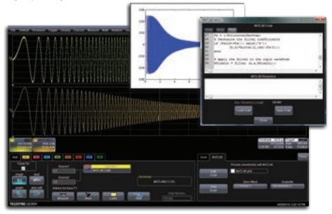
XDEV Customization software package being used to implement a 1 MHz Butterworth filter using MATLAB<sup>®</sup>.
