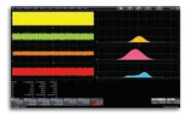
Capture a single clock channel (yellow) and display Track graphs and Histograms simultaneously of multiple jitter parameters.
