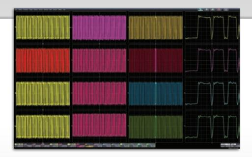
commonly used to synchronize lab equipment—ensures precise synchronization and high timebase accuracy between all acquisition modules. Additionally, a single trigger circuit for all modules eliminates additive trigger jitter that occurs with 10 MHz clocking and trigger synchronization of multiple conventional oscilloscopes.
