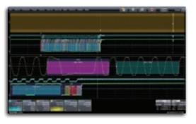
Capture 5 ms (100 Mpts) of low-speed and high-speed waveforms. Decode low and high speed serial data signals.Easily zoom, and validate timing relationships between signals.
