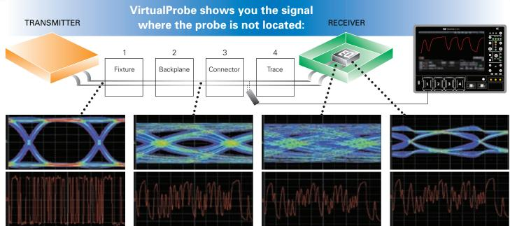
Virtually probe the signal at the transmitter with the fixture present, and then de-embed its effects form the measurement.
