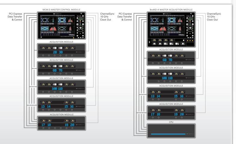
The LabMaster 9 Zi-A platform provides a modular, building block approach to minimizing initial investment while at the same time providing future flexibility. The minimum configuration is four channels at 13 GHz with maximum upgrade to 20, 40, or 80 channels at 45, 30, or 20 GHz respectively with up to 768 Mpts/ch of analysis memory.
