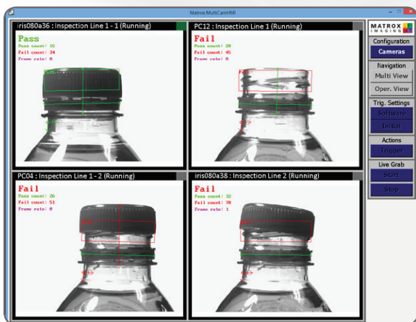
Multi-camera HMI application (Matrox MultiCamHMI)
