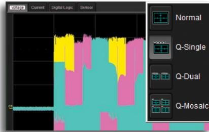
Use Q-Scape Multi-tab Displays to quadruple your display area. Customize tab names. Select from different Q-Scape displays (Single, Dual, Mosaic)
