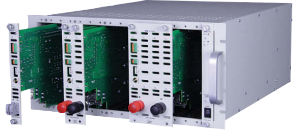
Front loading, card-based design makes removal & reconfiguration easy
