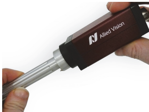
Figure 3: Removing IR cut filter/protection glass using special tool (E9020001)
