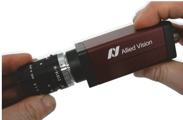
Figure 1: Illustration of camera orientation when removing lens or dust cap
