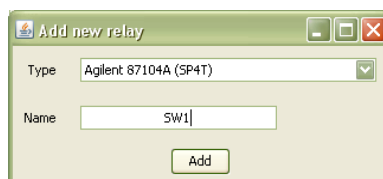
FIGURE A-6: ADDING AN AGILENT 87104A RELAY AS “SW1”
