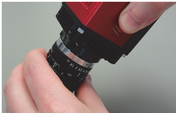
Figure 27: Illustration of camera orientation when removing lens or dust cap
