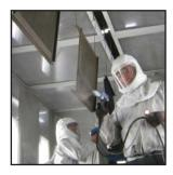
**Painting**We utilize a powder paint system that provides a high quality, durable and corrosion resistant finish. We also have e-coat capabilities if needed.
