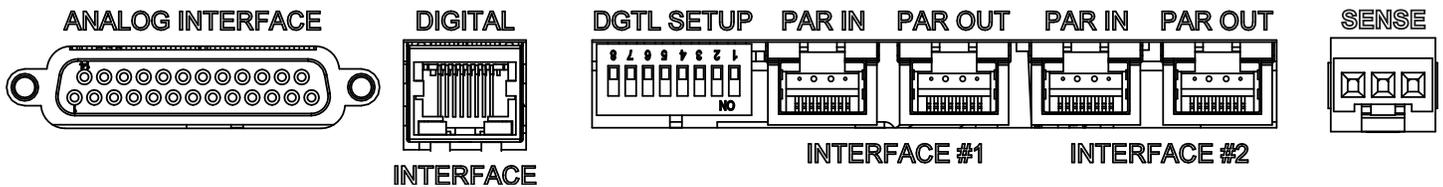
**Figure 2: External interface on the rear panel.**
