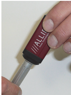
Figure 3: Removing IR cut filter/protection glass using special tool (E9020001)
